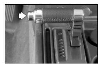
• Press the button on the end of the shift lever.
